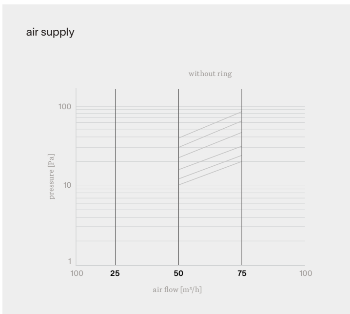
capacity graph - small cover plate
