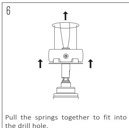
Pull the springs together to fit into the drill hole.
