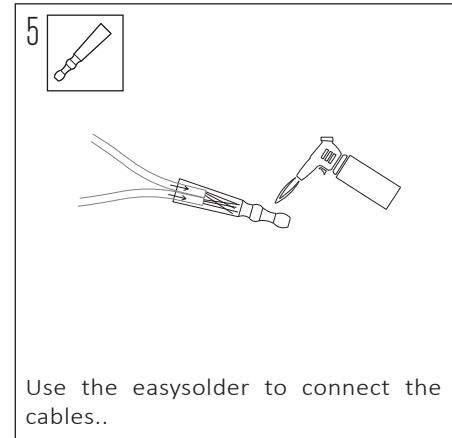
Use the easysolder to connect the cables..
