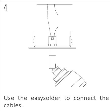
Use the easysolder to connect the cables..
