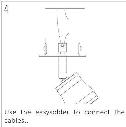
Use the easysolder to connect the cables..
