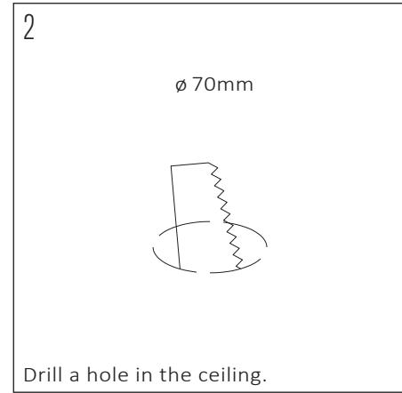
Drill a hole in the ceiling.
