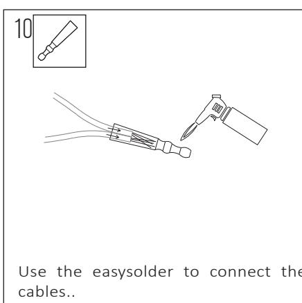
Use the easysolder to connect the cables..
