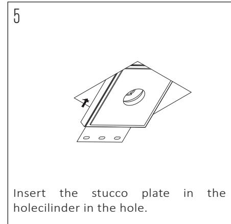
Insert the stucco plate in the hole cylinder in the hole.
