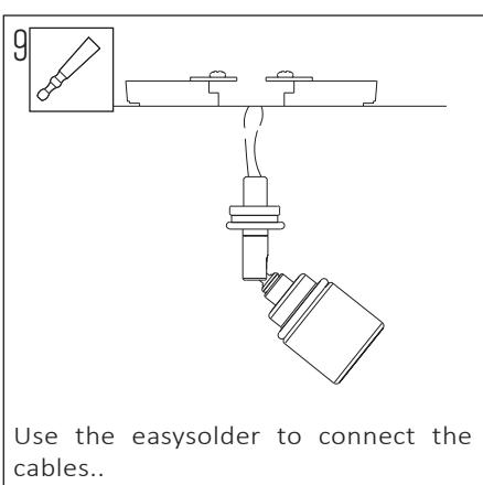
Use the easysolder to connect the cables..
