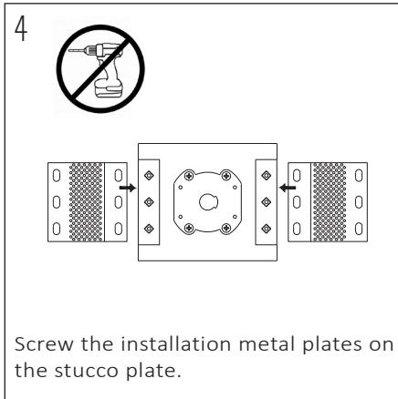
Screw the installation metal plates on the stucco plate.
