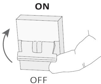
Be sure the installation is done right before switching ON the fuse.
