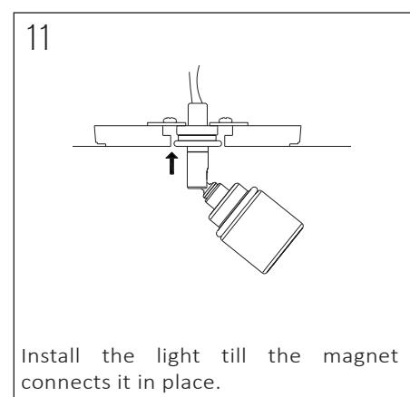
Install the light till the magnet connects it in place.
