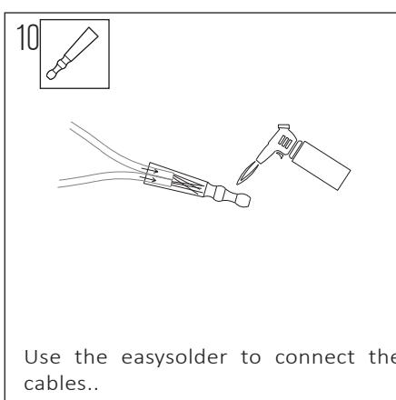
Use the easysolder to connect the cables..
