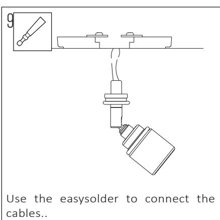
Use the easysolder to connect the cables..
