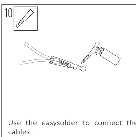
Use the easysolder to connect the cables..
