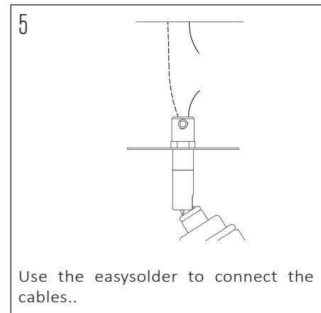
Use the easysolder to connect the cables..
