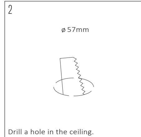
Drill a hole in the ceiling.
