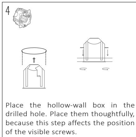
Place the hollow-wall box in the drilled hole. Place them thoughtfully, because this step affects the position of the visible screws.
