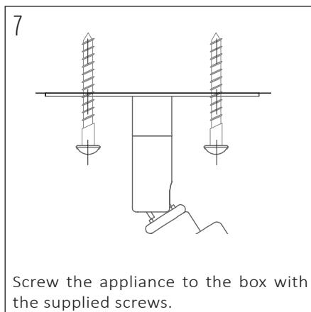
Screw the appliance to the box with the supplied screws.
