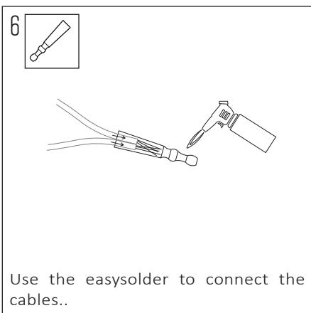
Use the easysolder to connect the cables..
