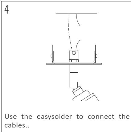
Use the easysolder to connect the cables..
