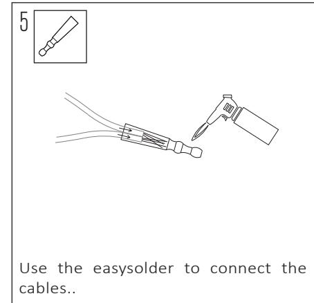
Use the easysolder to connect the cables..
