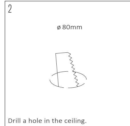
Drill a hole in the ceiling.
