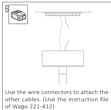
Use the wire connectors to attach the other cables. (Use the instruction file of Wago 221-412)
