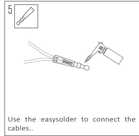
Use the easysolder to connect the cables..
