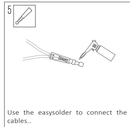
Use the easysolder to connect the cables..
