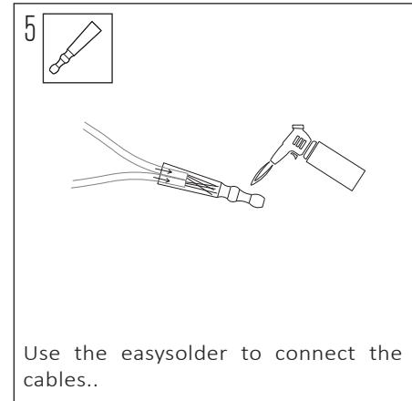
Use the easysolder to connect the cables..
