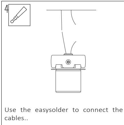
Use the easysolder to connect the cables..
