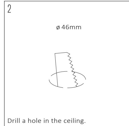
Drill a hole in the ceiling.
