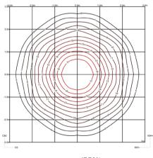
Efficiency Coordinate System Total Flux Maximum Value 47.70% CG 1920.00 lm 88.28 cd/klm
