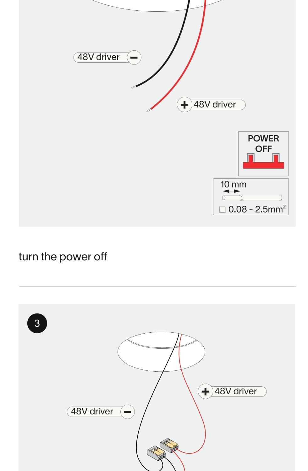
connect the wires with wago connectors
