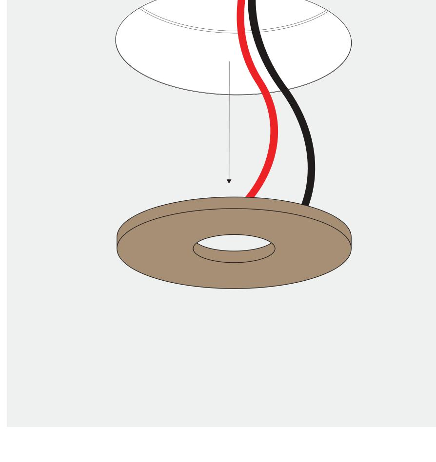
Remove the plaster lid before installing the fixture. Any residue needs to be removed without damaging
