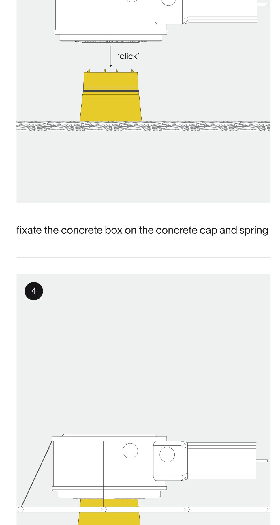
strongly attach the concrete box to the reinforcement
