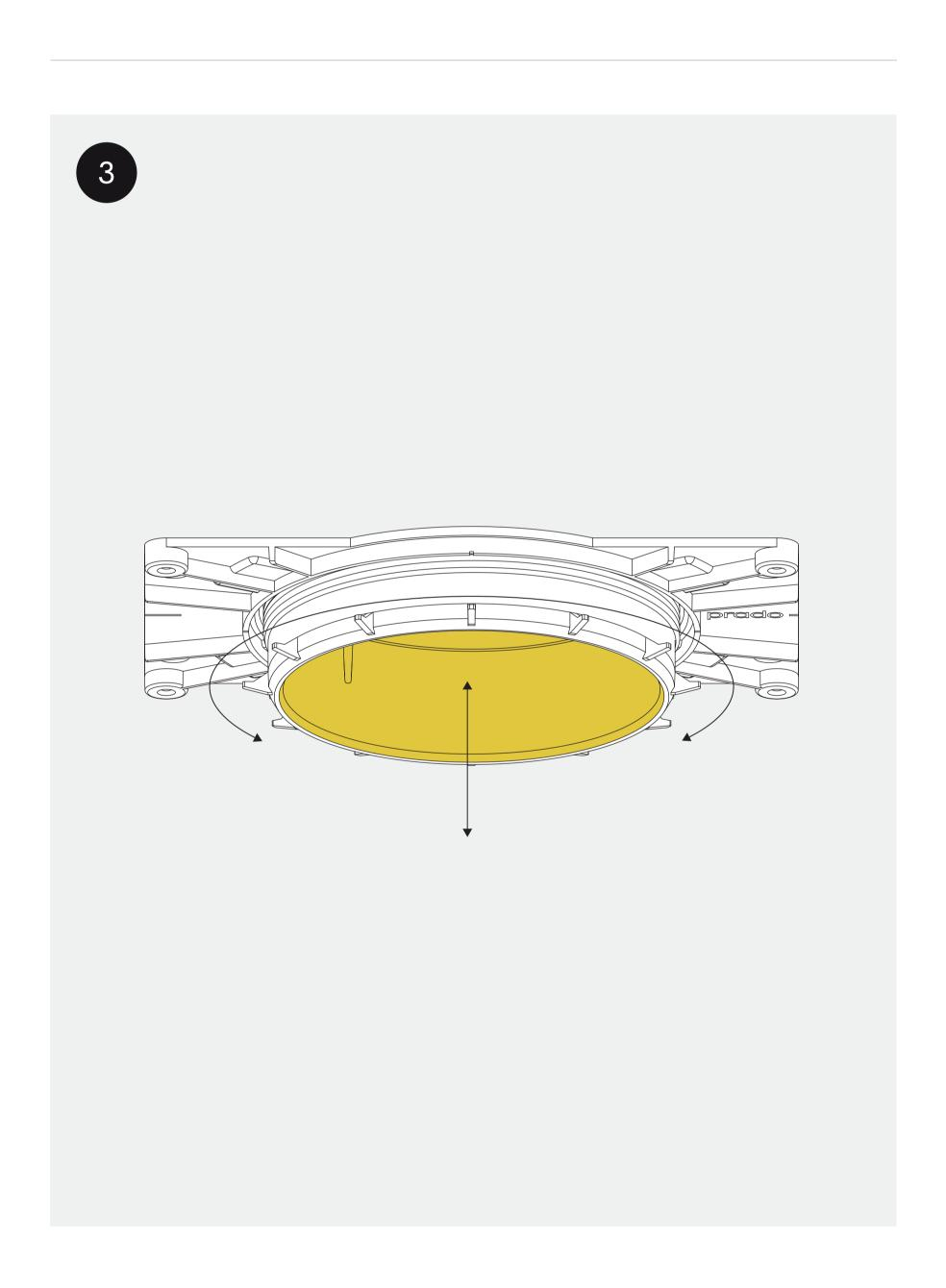
Adjust the height of the plaster ring by twisting the bottom part.
