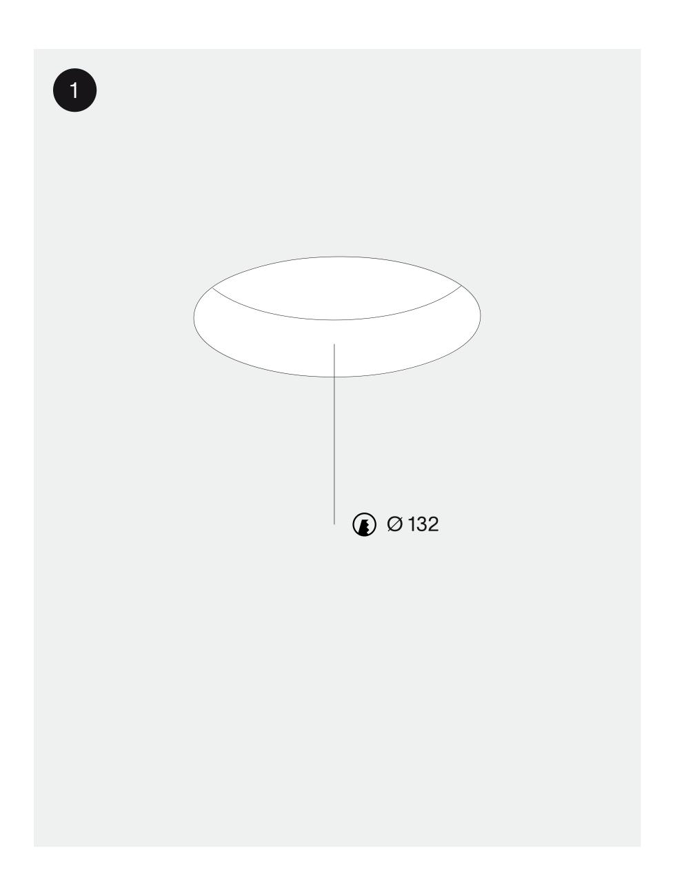
Cut a round hole (Ø 132). Consult the chosen luminaire tech specs for required height and free air dimensions.
