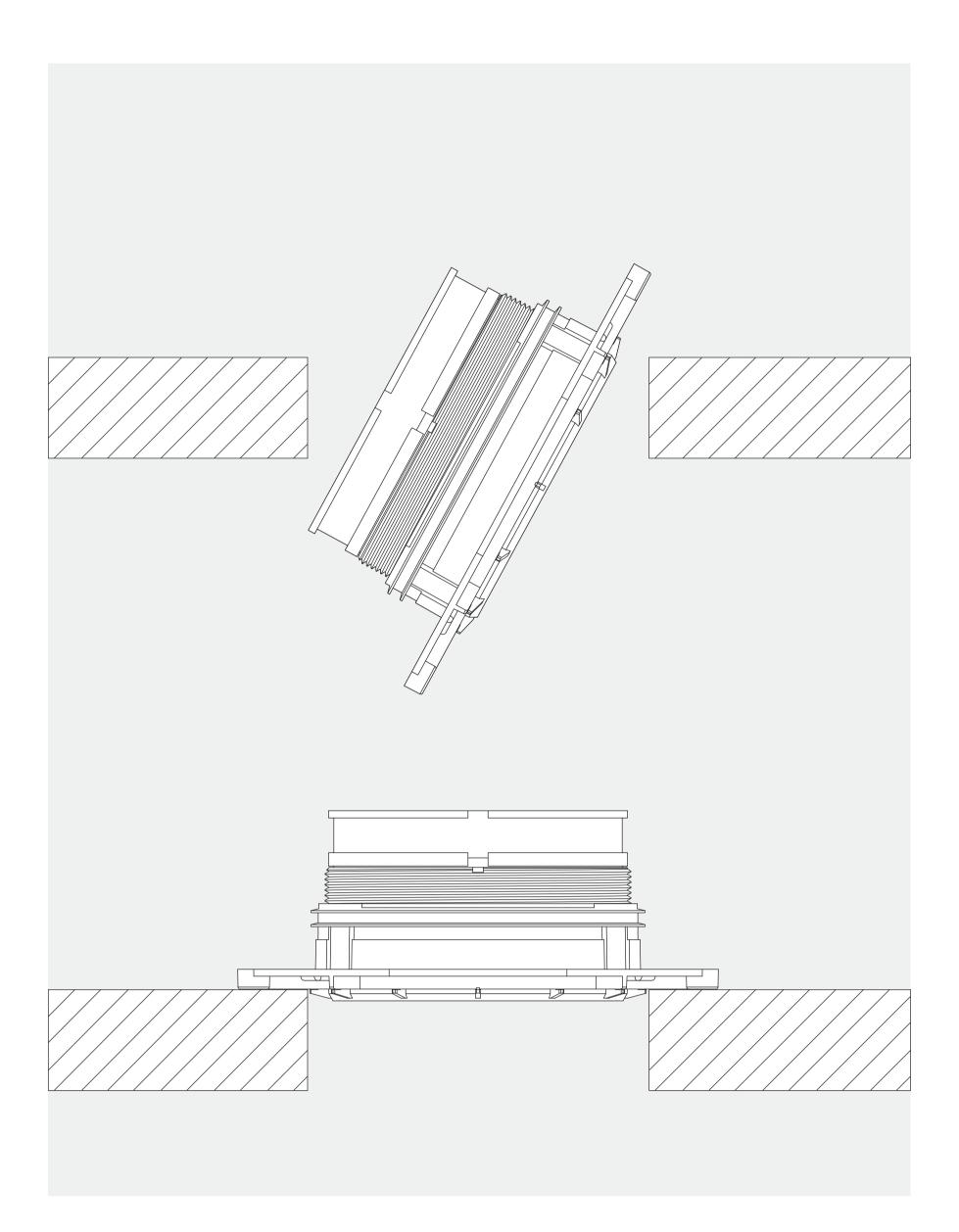
Slide the plaster ring through the Ø132 hole to install on top of the ceiling.
