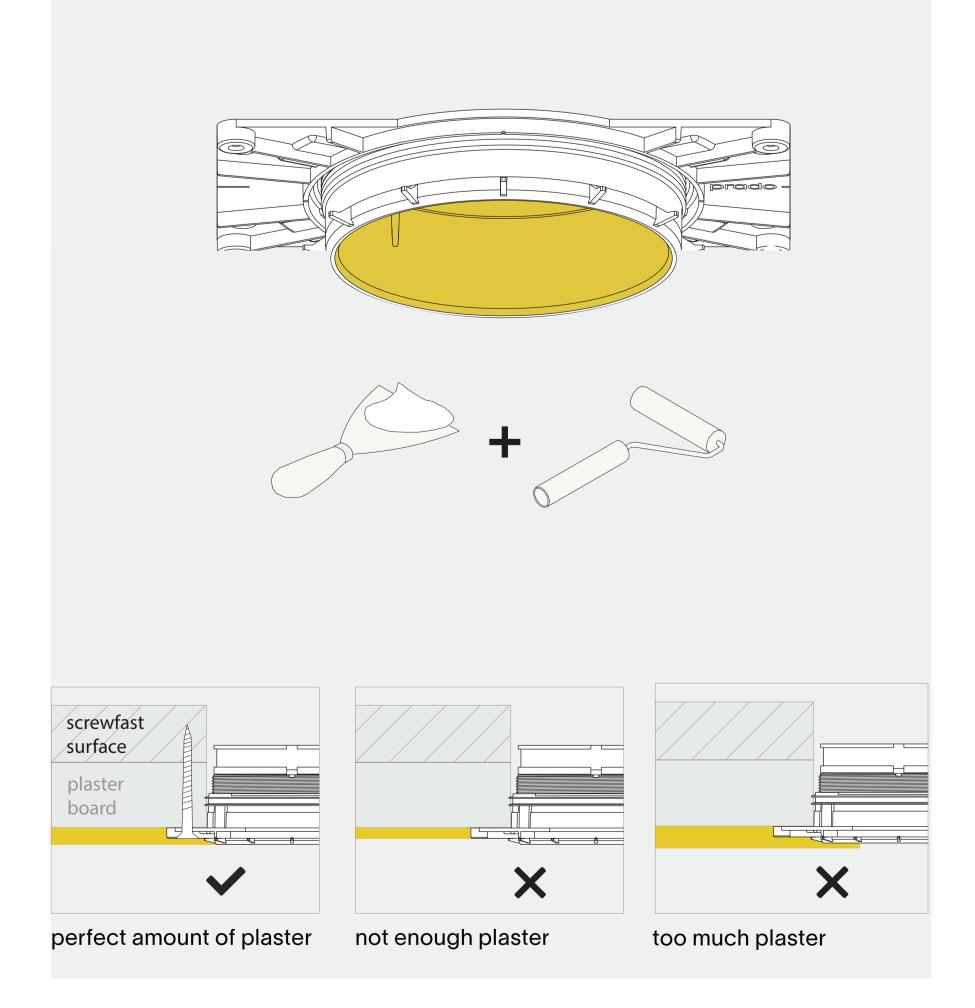
Excercise caution while plasering, do not damage the ring. Keep the plaster lid inside the plaster ring while plastering. Use a fiberglass mesh tape for optimal plaster adhesion. Make sure not to touch the edge of the ring when sanding.
