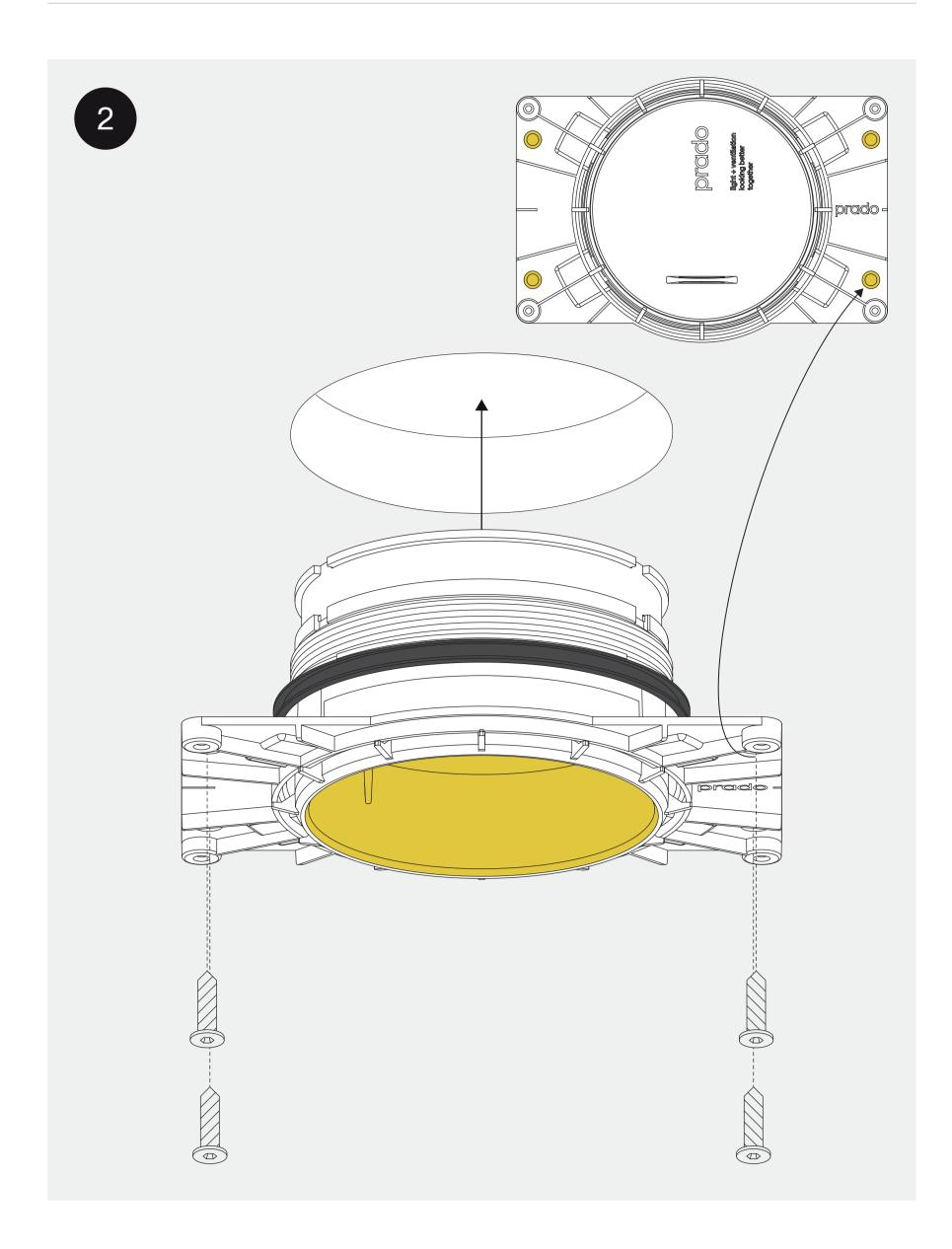
Insert the plaster ring and securely fasten it with glue or the appropriate screws on a screwfast surface. The attachment must be able to obtain a static load of 5 kg. It's the installers responsability to ensure optimal attachment.
