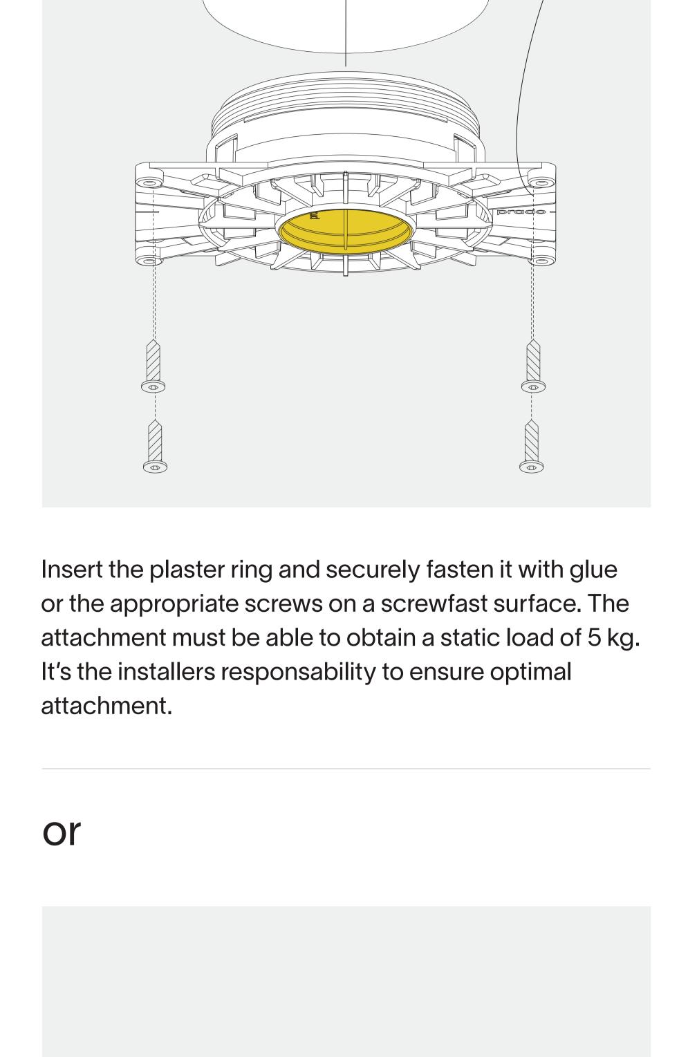
Slide the plaster ring through the Ø132 hole to install on top of the ceiling.
