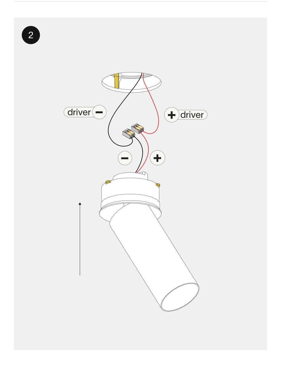
connect the wires with wago connectors
