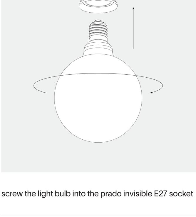
screw the light bulb into the prado invisible E27 socket
