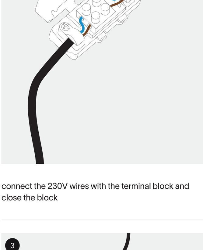
connect the 230V wires with the terminal block and close the block
