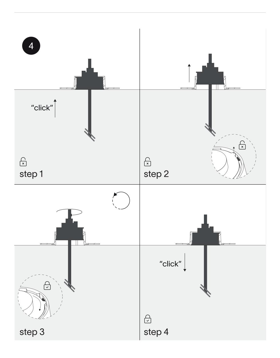
Insert the luminaire into the ceiling until it "clicks". Push the luminaire a little further and twist it to lock it. Gently pull the luminaire down again. Now it's locked.
