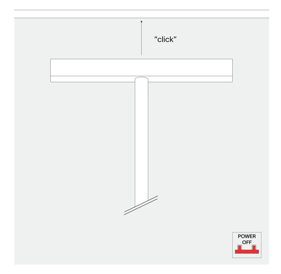
slide pendant track adapter in the prado 48V track and make sure a prado 48V LED-driver is used for the track pendant cable length cannot be adjusted after delivery
