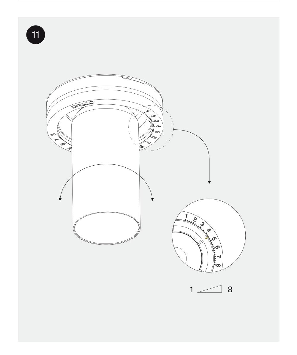
twist the luminaire to adjust the ventilation flow level
