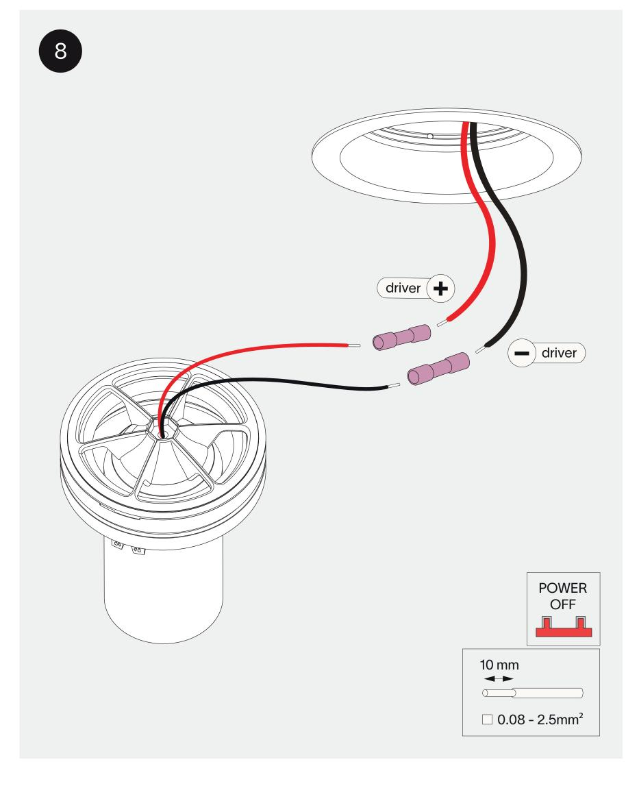
connect the wires with waterproof connectors for serial connection, respect polarity combine with prado LED-driver
