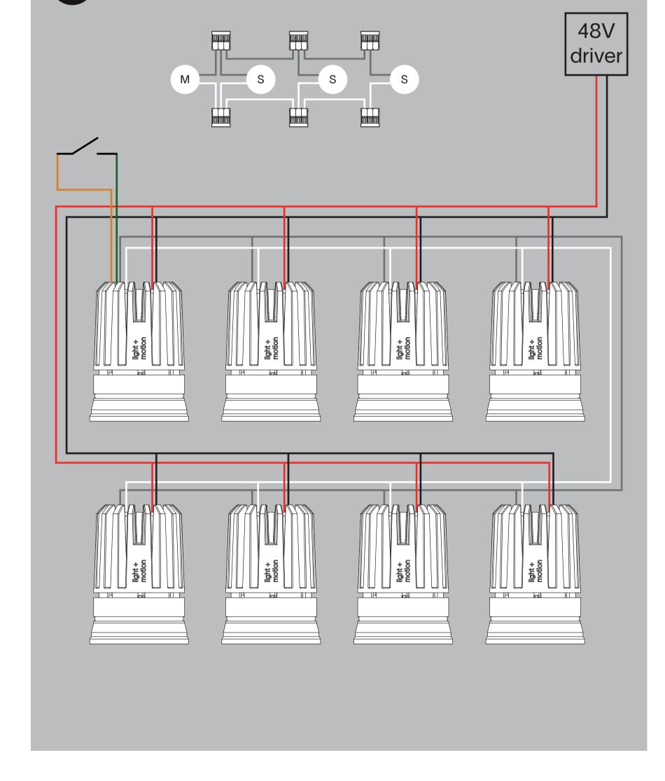
all master/slave modules must be powered by one driver
