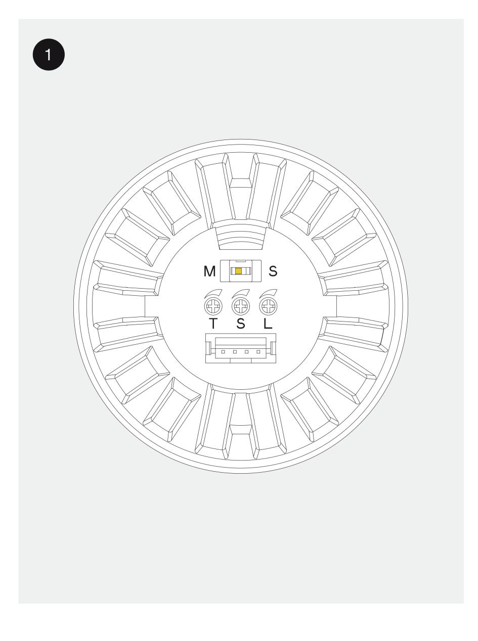
set the luminaire in master or slave mode with the switch (1 = master - rest = slave)
