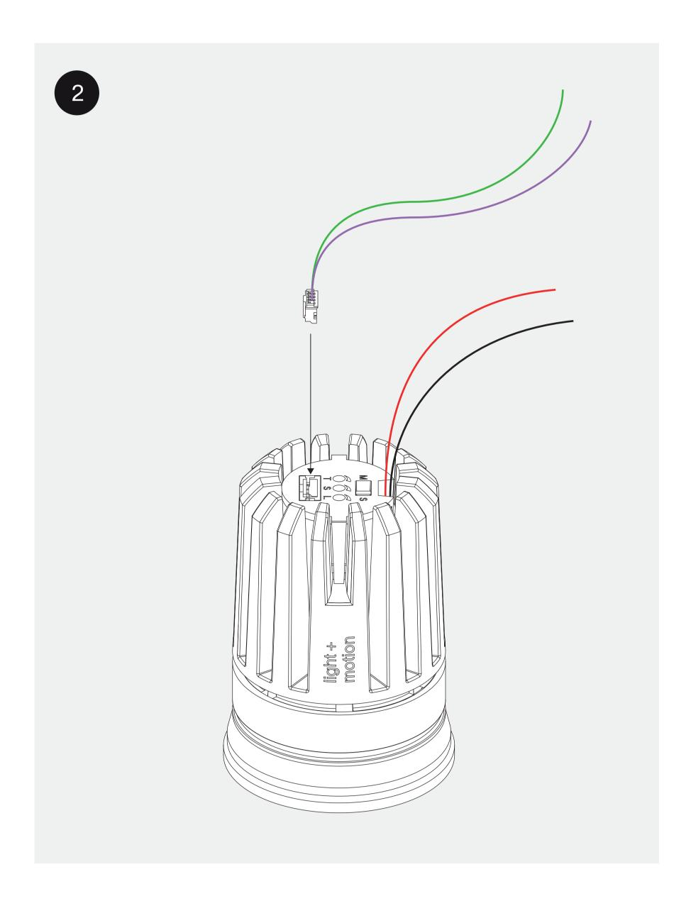
set the luminaire in master or slave mode with the switch
