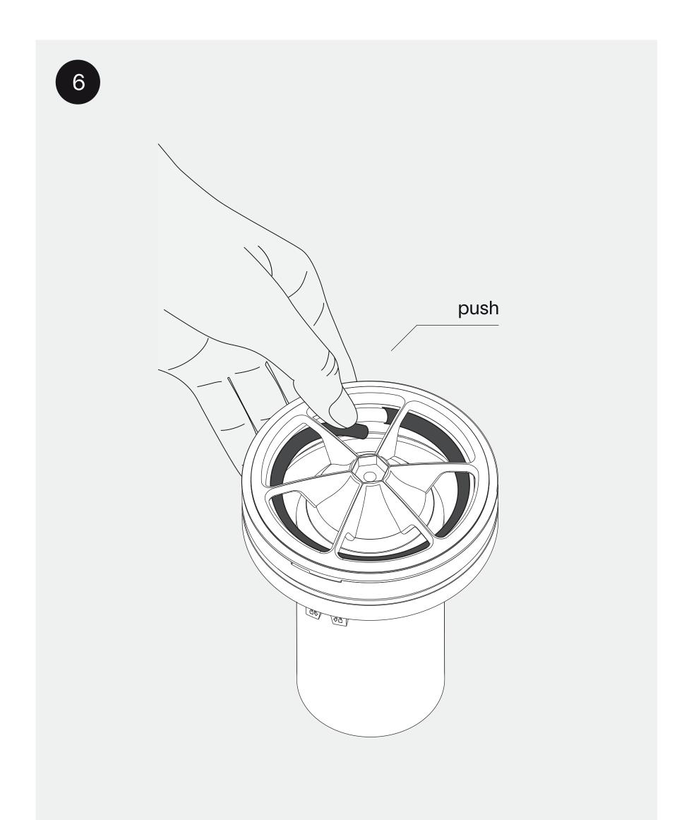
if 50m³/h is required remove the 25m³/h ring like shown above
