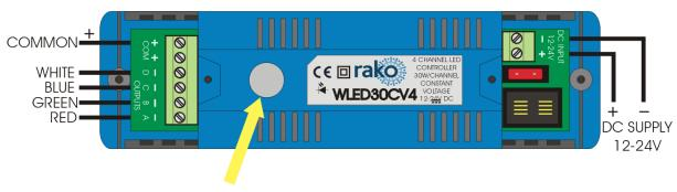
NOTE: WHITE WILL NOT BE USED ON 3 CHANNEL TAPE SET-UP BUTTON AND MANUAL ON/OFF
