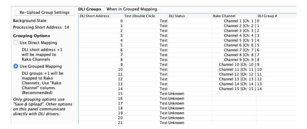
It is possible to test which ballast is associated to which short address by using the test column on the mappings page. Double click on "test" to send and "on" to this ballast, double clicking again will send an "off." When an "on" is successfully sent the row will appear as below.
