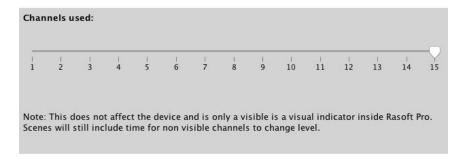
Slide the "channels used" slider to match the number of Channels required by the WSR-DLI and the remaining channels are freed up to be used by other devices.
