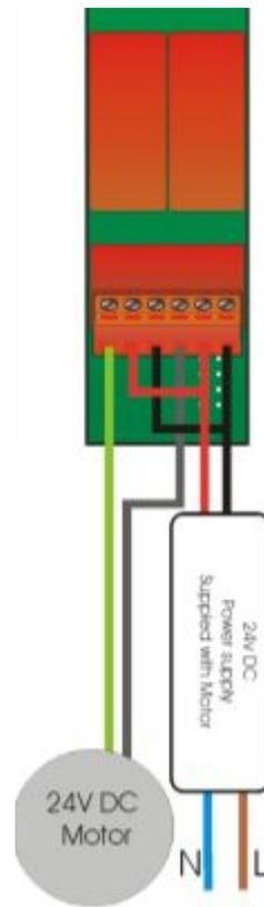
**Contact closure blind wiring diagram:**
