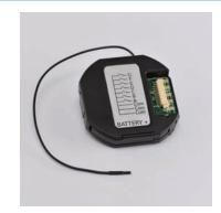
The RCI-7M accepts volt-free momentary switch inputs and transmits wireless Rako coded Rakom messages to other Rako wireless receiver and Bridge units. The module is battery powered and is designed to fit in a standard UK backbox.
