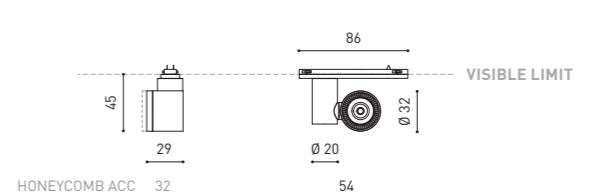
COLOUR | WT □ RAL 9016 | NT ■ RAL 9005 | MATERIAL | AL | OPTICAL PMMA |
