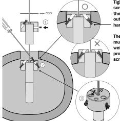
Tighten the screws until they bottom out on the hardware.
