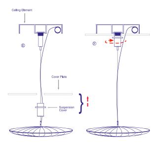
The lamp is hung leveled by default (position A). If you wish to install the shade on an angle, tilt the lamp to the desired position (position B) and then tighten the 3 screws as marked in figure 1 to lock the position.
