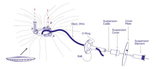
Install the O-ring by tightening the screws shown. Then loosen the 2/1 a turn counterclockwise to allow an almost non-friction movement of the ball.
