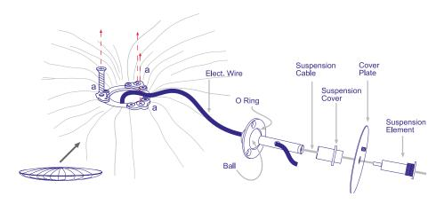
Install the O-ring by tightening the screws shown. Then loosen the 2/1 a turn counterclockwise to allow an almost non-friction movement of the ball.
