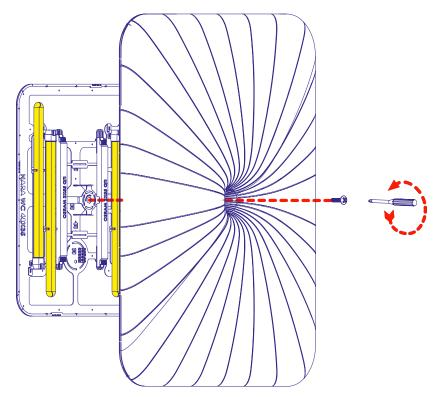
5. Push supplied stainless steal plate with the magnet as shown.
