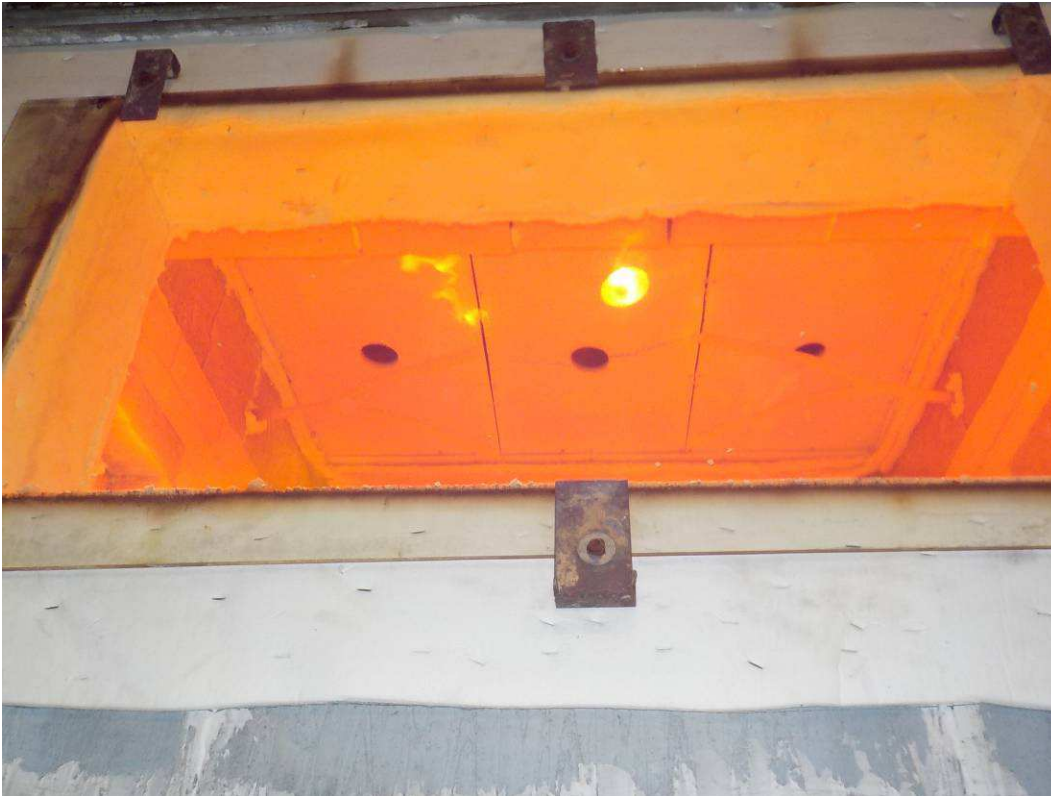
Photo 2.2.5 – Exposed face after 60 minutes.
