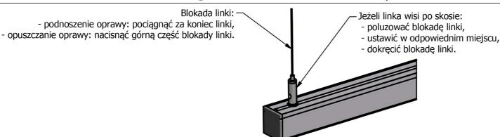
Set the luminaire to the appropriate height and level it with the cable lock.
