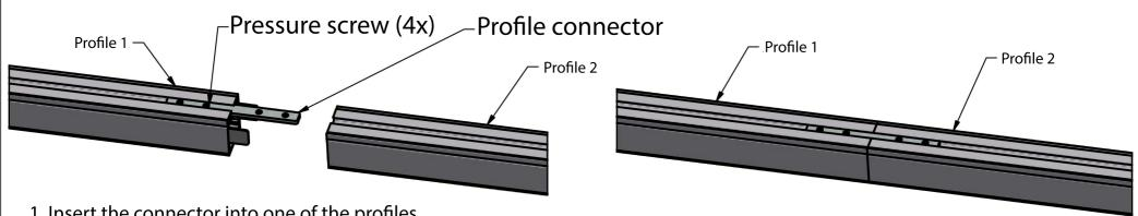
1. Insert the connector into one of the profiles, tighten the two grub screws.
