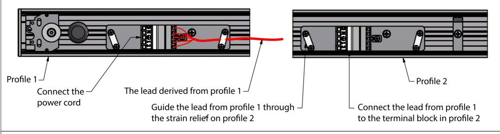
8. If the cartridges have been completely dismantled, attach them to the safety devices again. Connect the supply cord to the closest terminal block. Insert the insert into the profile so that it adheres to the magnets, the element positioning the insert should hit the hole in the magnet plate.
