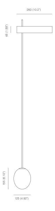
Bulb specifications 120V / 240V G9 3,5W LED Bulb 350Im / 2700K
