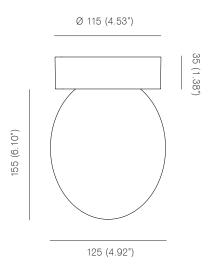
Bulb specifications 120V / 240V G9 3,5W LED Bulb 350Im / 2700K
