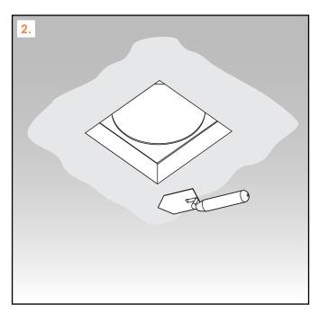
If the powder coat gets damaged during installation the kits must be resealed with a rust proof solution before continuing to skim with plaster.
