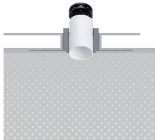
The Moon range of trimless, recessed fixtures matches utmost performance to incredible compactness. Recessed optics ensure high visual comfort. Revolutionary in dissipative, functional design, it offers the possibility to combine colour temperatures and beam angles in CRI85 and CRI93 and CRI98 with R9 93 versions.
