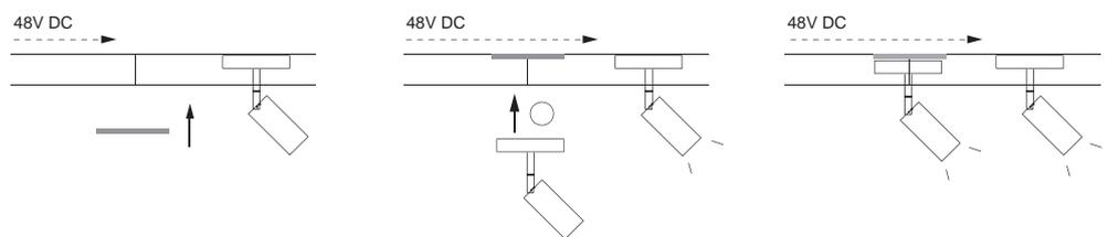
Use the joint 10-CDS to connect the tracks
