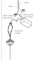
Connect the house wires to the coaxial cable using #16 butt splices (stagger the splices). Use raw butt splices and heat shrink to simplify the installation.
