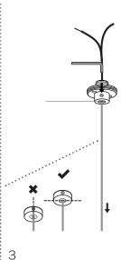
Thread the coaxial cable through the canopy. Throughout installation be mindful not to damage the borosilicate tube
