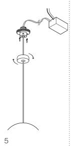
Affix mini-canopy to ceiling surface with fasteners provided. Twist the threaded canopy cover plate into place.
