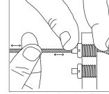
7. Adjust the height of the lamp by pressing the wire griper and then, cut the excess wire, as shown.
