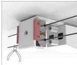
6. Insert the + wire in the + terminal and the - wire in the - terminal.
