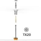
2. Drill holes and fasten the plastic ceiling components.
