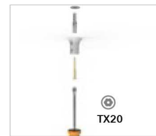
2. Drill holes and fasten the plastic ceiling components.
