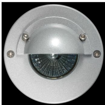
The Step Lite Eyelid is designed with a 88mm (3 1/2") flange and recessed body for flush mounting into masonry, stone or wood, providing illumination of steps and low level features such as exterior paved areas. The Eyelid feature eliminates all upward light, providing an excellent glare-free illuminating effect. When a canister is used there are no mounting holes in the flange.
