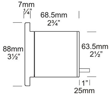
The Step Lite is designed with a 88mm (3½”) flange for flush mounting into masonry, stone or wood. This luminaire is ideal for illumination of steps and ground level horizontal lighting, for example, across driveways or exterior paved areas. When a canister is used there are no mounting holes in the flange.
