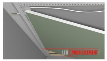
**12.** Make a large notch in the gypsum board to allow access for the supply cable.
