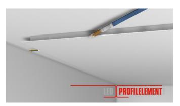
**27.** Lightly smooth and remove surplus paint or other undesired material from the edges of the profile.
