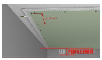
**15.** Fix screws along the edges of the profile. If necessary, cut off any screw tips that stick out of the back of the profile.
