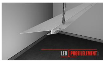
**04.** Drill the opening for the LED connecting electrical cables from above with a metal drill bit.
