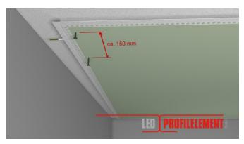
**14.** Screw the gypsum boards to the profiles leaving 150mm between each screw.
