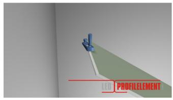
11. Cut the gypsum boards to size and slide into the profiles.
