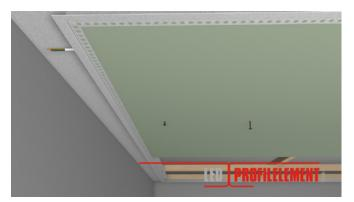
**13.** Screw down the gypsum boards according to the manufacturer's instructions.
