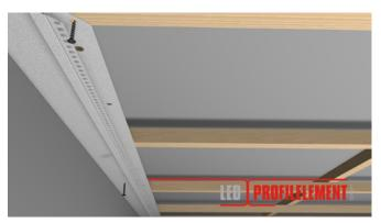
**09.** Screw the profile to the framework using regular gypsum plasterboard screws.
