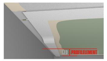
**18.** Attach the paintable fleece to the slotted metal profile in small strips with a brush and cold glue. Observe the drying time stated by the adhesive manufacturer.
