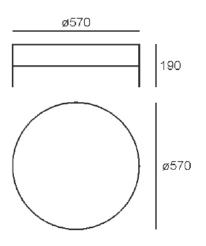
Cable length: 1200mm Ø570mm H.190mm
