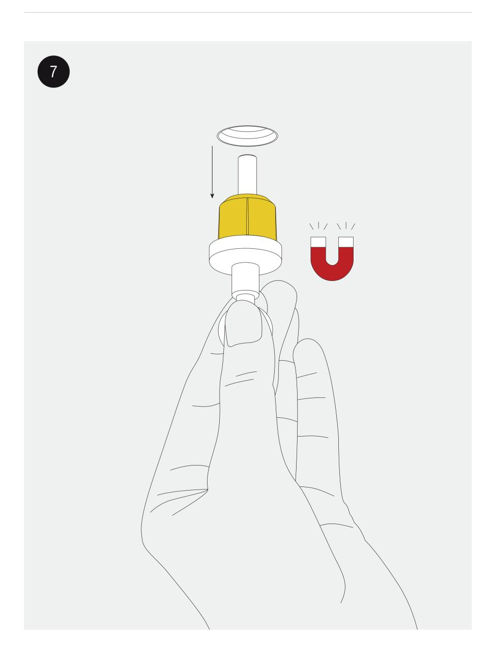
Remove the plaster lid with a magnet before installing the fixture. Any residue needs to be removed without damaging the edges of the installation ring.
