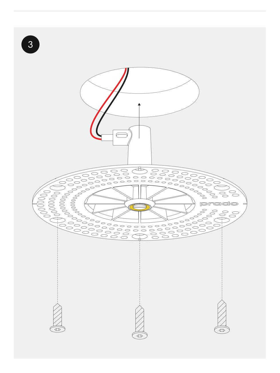
Insert the plaster ring and securely fasten it with glue or the appropriate screws on a screwfast surface. The attachment must be able to obtain a static load of 5 kg. It's the installers responsability to ensure optimal attachment. We advise to test the electrical connection before starting to plaster.
