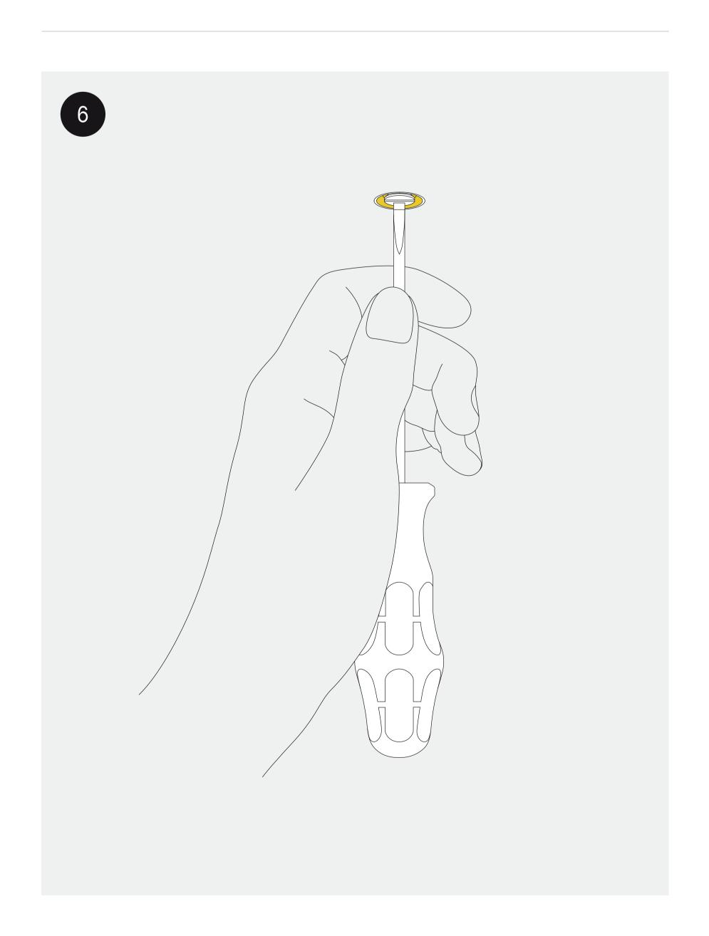
Twist the yellow plaster lid with a screwdriver before removing it with a magnet.
