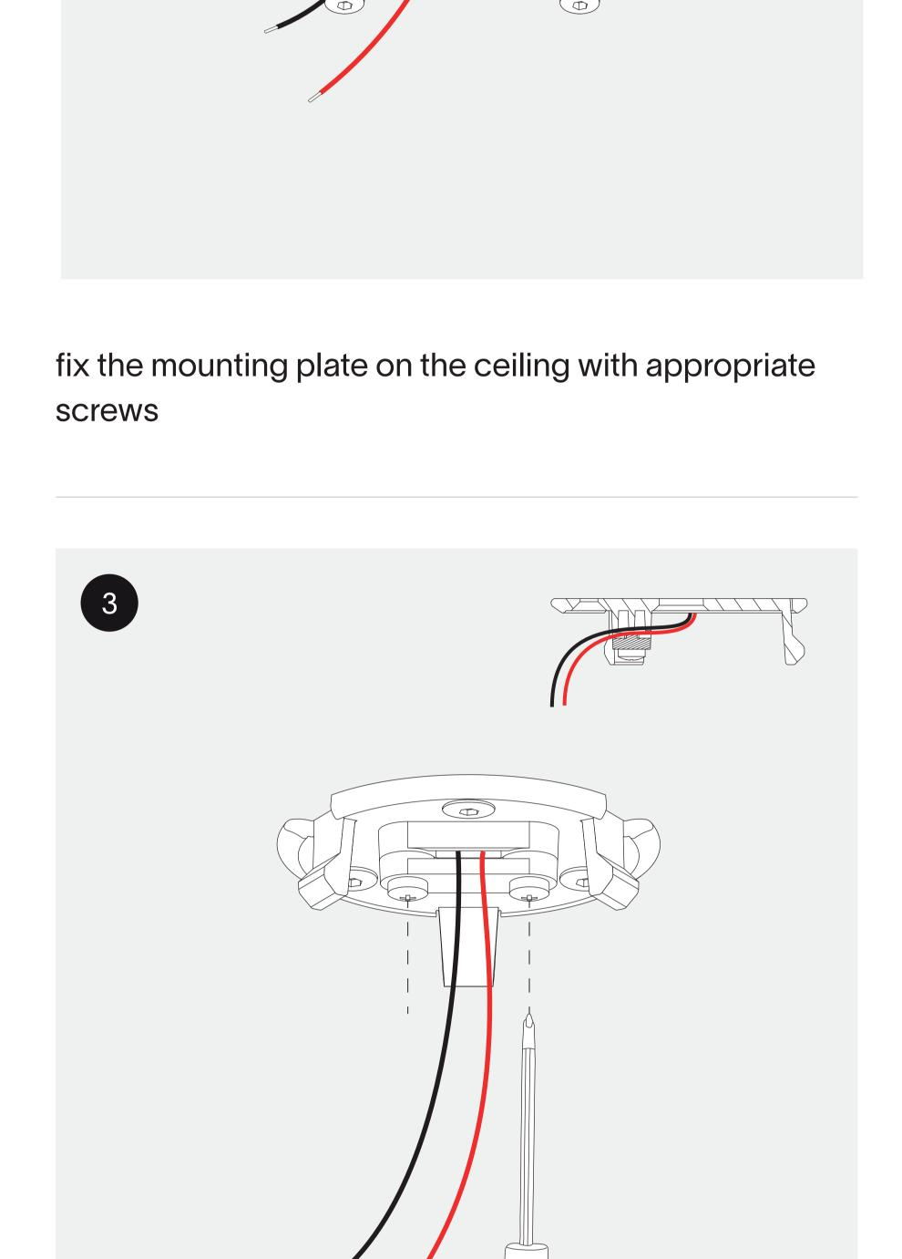
tighten the wires through the strain relief and cut off the
