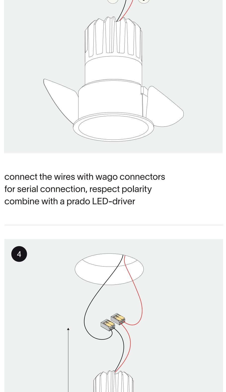
bend over the springs and push the luminaire into the
