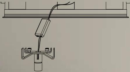
Wire the product and pass the power supply through the side holes of the duct.
